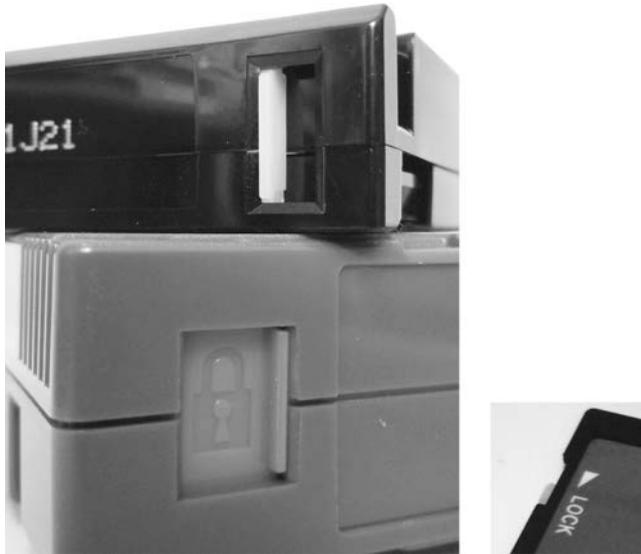
Figure 4-5: Write-protect tabs on tapes and SD cards
