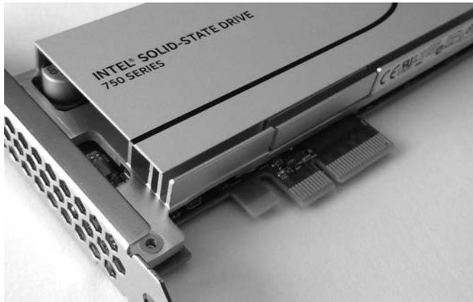
Figure 1-16: NVME SSD with a PCIe interface
