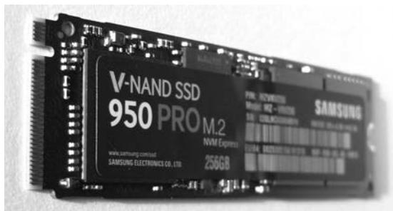
Figure 1-17: NVME SSD with an M.2 interface
