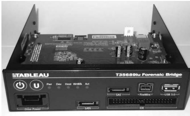
Figure 4-2: Multifunction drive bay write blocker
