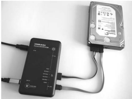
*Figure 4-1: Portable SATA write blocker*
