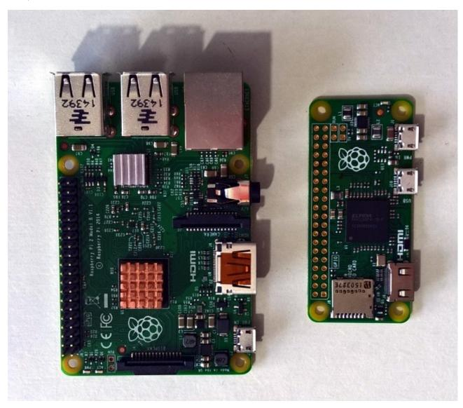
Less than half the size of the traditional Raspberry Pi, it's even-more-compact dimensions make it ideal for projects that require a board that can slip into small gaps, as well as one for which weight is a consideration. For example, the Raspberry Pi 2 weighs 45 g (1.6 oz); in contrast, the Pi Zero is just 9 g (0.32 oz).
