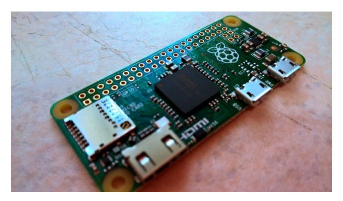
Finally, a MicroSDHC slot is provided, for high storage disks with robust error-connection, while the GPIO is – in a Raspberry Pi first – unpopulated, which means you need to solder your own pins onto the Pi Zero. Among the "missing" components, you'll find that there is no video input for the Raspberry Pi camera and NoIR camera modules.
