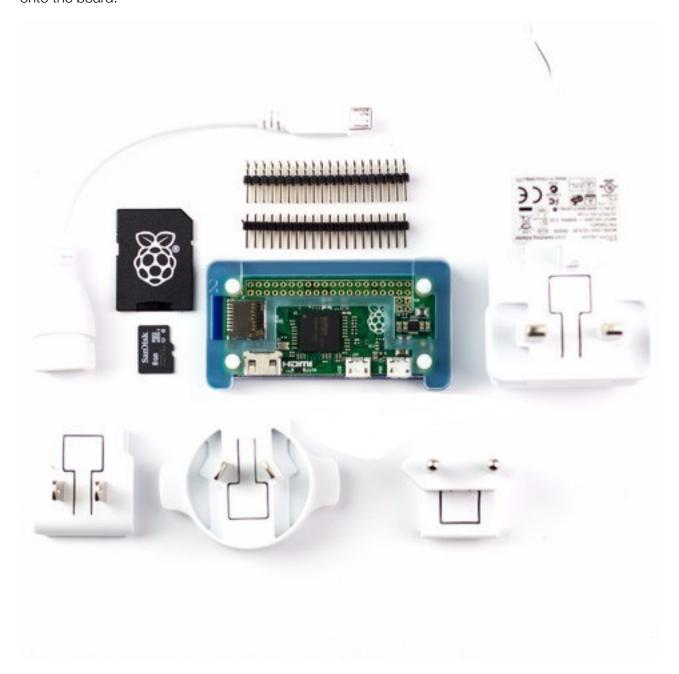
You will also find a more modest kit, like that shipped on the cover of MagPi magazine, offering the Mini HDMI adaptor, USB OTG cable, GPIO header pins, and little else.
